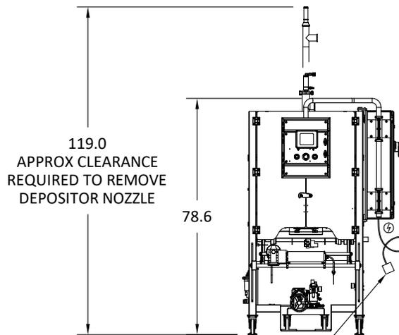
7' CORD W/ NON-NEMA, WATER TIGHT, 20A, 120/208V, 3 PHASE, 4 POLE, 4 WIRE PLUG (CONNECTING FEMALE RECEPTACLE INCLUDED)
